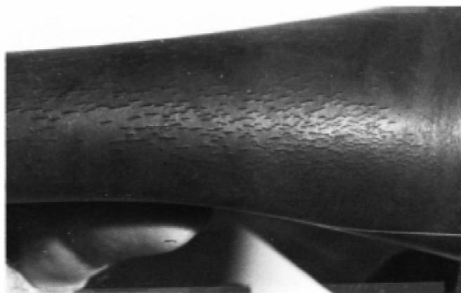
FIG. 18 Ozone Cracks
